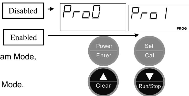
Press the ▲ button to enable Program Mode, “Pro1” and “PROG” are displayed.
