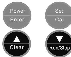
When pump display matches reference meter press SET button.
