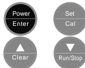
Press ▲ button to increase flow rate set point or ▼ button to decrease flow rate set point, in 0.01 L/min increments.
