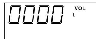
When the data is cleared, the AmpHr accumulator is cleared so that starting a new run will correctly display remaining battery capacity. When the data is cleared, the pump should be charged.
