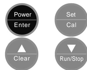
When desired flow rate set point is reached press ENTER button. Pump will return to Ready Mode. Elapsed Time and Total Volume will be cleared
