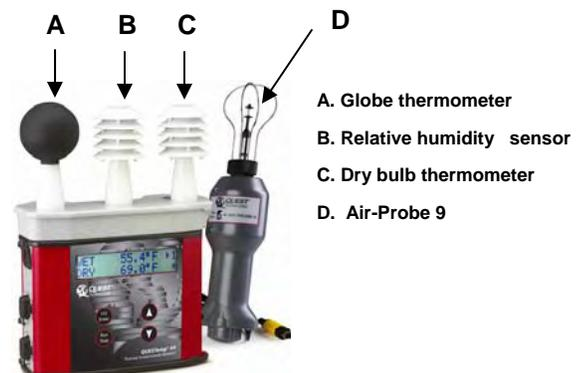
Figure 1: QUESTemp<sup>o</sup> 46 with Air-Probe 9
