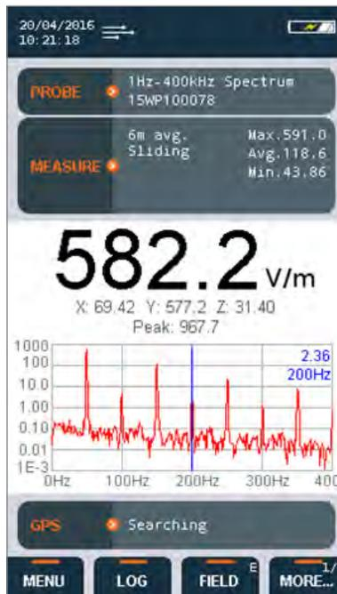
Figure 1. Evaluation of harmonics by spectrum analysis
