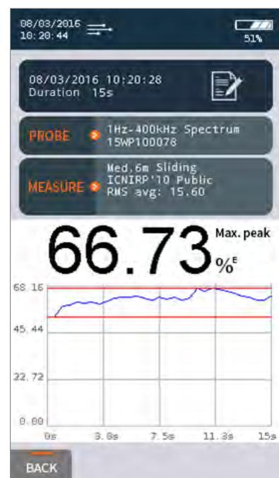
Figure 8: SMP2 screen in weighted peak mode
