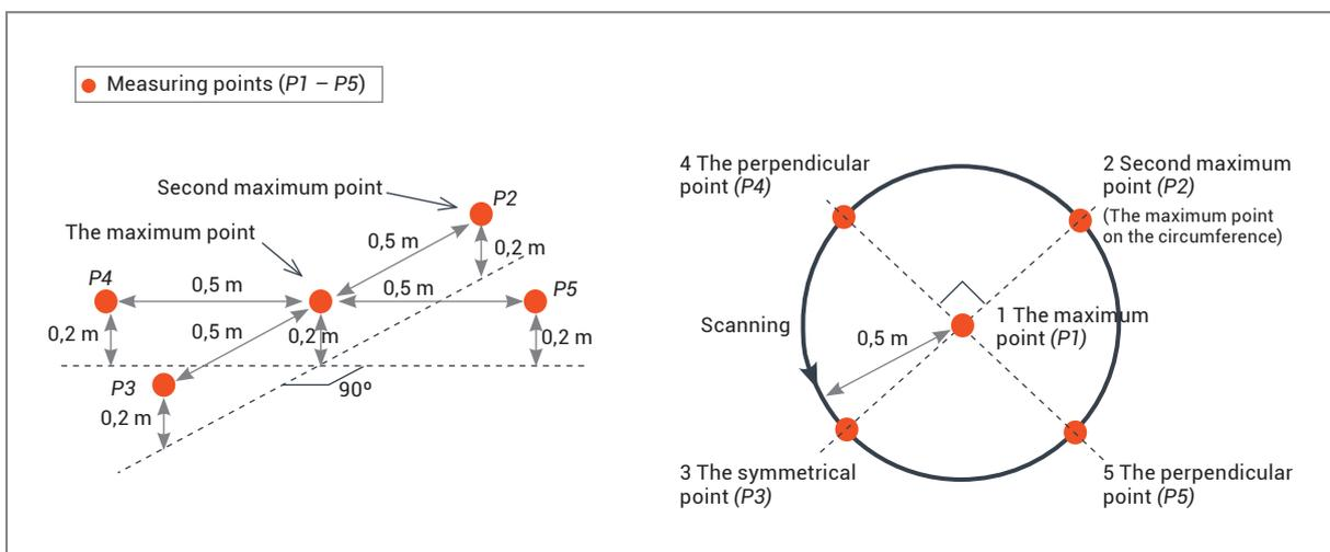
Figure 5. Points for the spatial average over a field source
