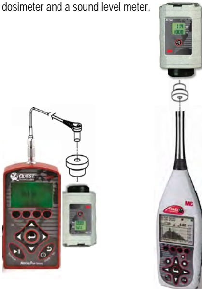
Figure 4: Examples of performing a calibration
