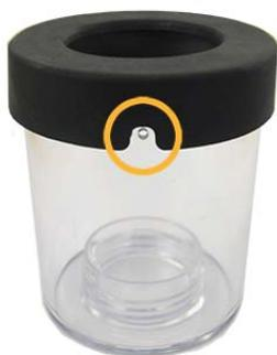
5. Fill the cup to the fill line with calibration standard. Place the instrument in the calibration cup and select **Next**.
