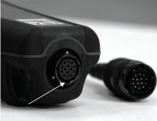
Figure 4, Note the keyed connector.
