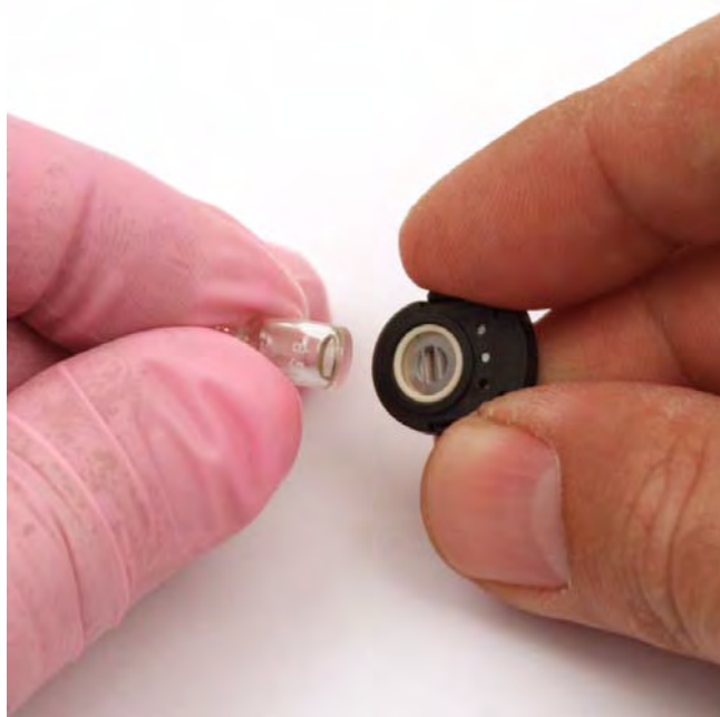
Figure 32: Reinstalling the Electrode Lamp
