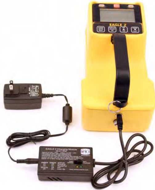
Figure 15: Connecting the EAGLE 2 to the Charger
