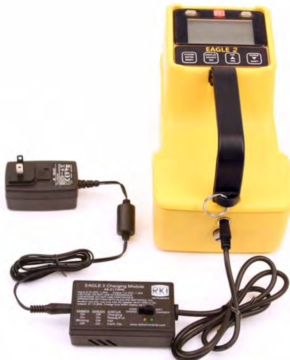
Figure 18: Connecting the EAGLE 2 to the Charger
