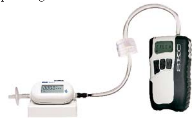
Calibration train with sample medium in line
