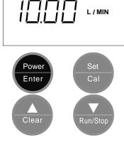
Press ▲ button to increase flow rate set point or ▼ button to decrease flow rate set point, in 0.01 L/min increments.
