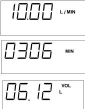
If no buttons are pushed, Ready Mode continues cycling through screens for 75 minutes then pump turns off.
