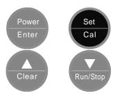
Press ENTER button to enter Calibration Mode. "SCAL" (Self-Calibration) is displayed for 10 seconds, allowing the pump to establish a zero reference for the flow control system. Pump will then start running, and display the set flow rate.
