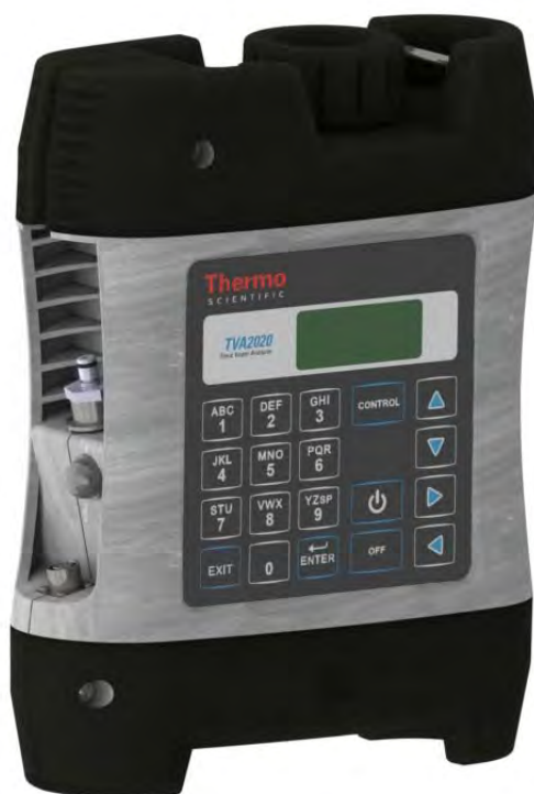
Figure 2–1. Instrument Sidepack Display
