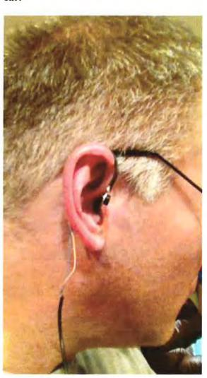
Don earmuffs over ear clip allowing the thin wires under the muff cushion. The thin wires have negligible effect on earmuff performance.
