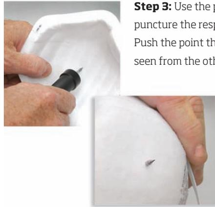
**Step 3:** Use the piercing tool to puncture the respirator from the inside. Push the point through far enough to be seen from the other side.
