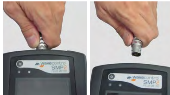
Figure 9: How to disconnect the field probe
