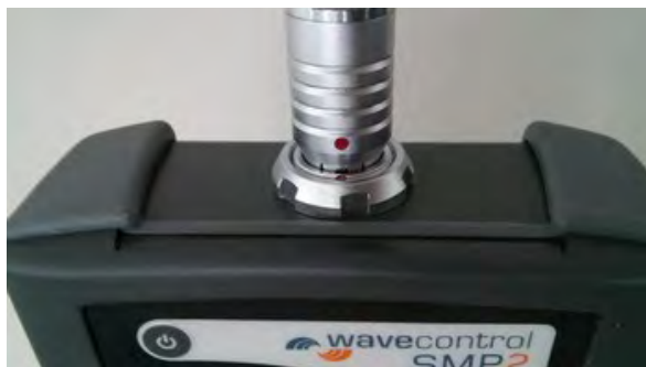
Figure 8: How to connect the field probe
