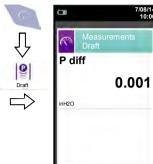
Before zeroing the pressure it is mandatory to REMOVE the probe from the chimney.
