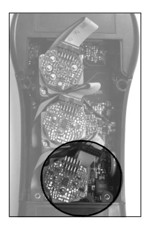
The sensor is bayonet-connected to its socket; rotate it counter-clockwise to remove it. Here is an example of a rotated sensor.
