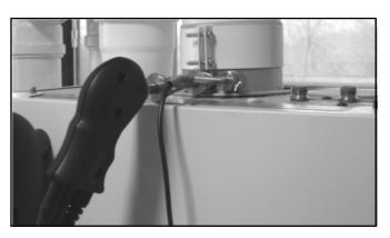
The screw on the cone allows the probe to be stopped at the right measuring depth - this usually corresponds to the center of the exhaust pipe. For greater positioning accuracy, the user may insert the probe gradually into the pipe until the highest temperature is read. The exhaust pipe must be inspected before carrying out the test, so as to ensure that no constrictions or losses are present in the piping or stack.
