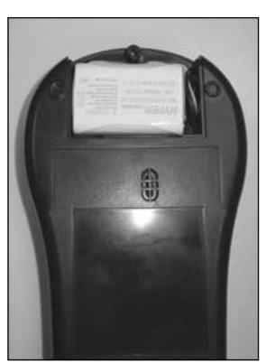
Remove the battery pack connector, and replace the pack with a new one following the reverse procedure described above.
