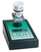
Bio-Pump with Bioisolation filter
