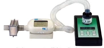
Bio-Pump connected to a TSI Primary Flow Calibrator
