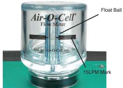
Adjust flow until ball is centered on line.
