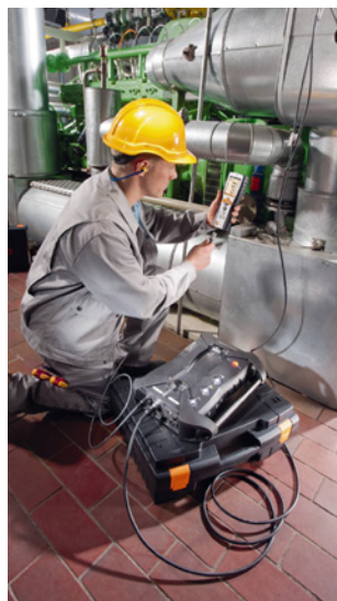
Figure 43: testo 350 – flue gas analyzer system for industrial emissions measurement
