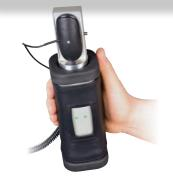
In-situ checks require to use a vibration calibrator such as the SV110 and are intended for checking the instrument's basic calibration and functionality in the field. During the check procedure, the SV107 accelerometer is mounted on the shaker with the SA105A calibration adapter and is excited at vibration level of 10 m/s<sup>2</sup> at 80 Hz. The check procedure lasts 30 s for each axis.
