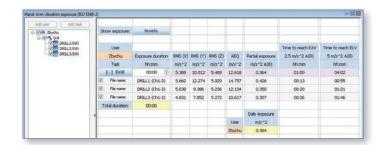
The Supervisor software automatically calculates A(8) vibration exposure value for the time that the contact force was detected. The tools provided with the SV103 enables the user to project the working time with the vibrating equipment as well as removing artifacts from the A(8) calculation. Reports are done in MS Word<sup>TM</sup> format and can be generated with a single click.
