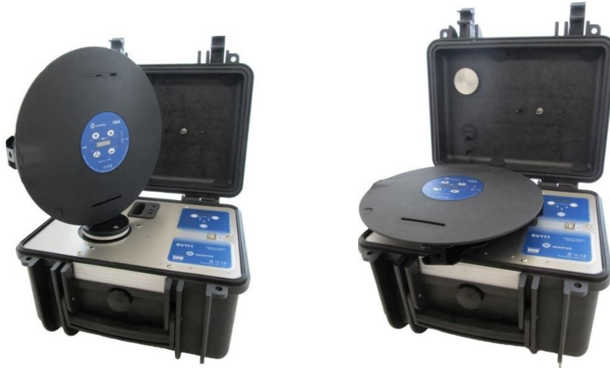
Figure 4-6 Using the SV 111 calibrator
