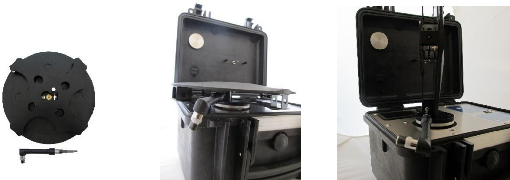
Figure 4-6 Calibration with SV 111 calibrator
