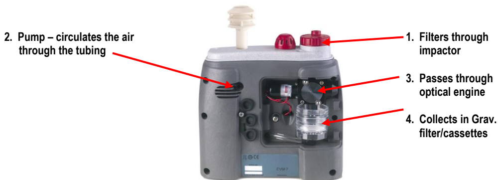
Figure 4-3: How the impactor functions
