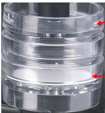
Figure 7-10: Gravimetric cassette and filter paper maintenance
