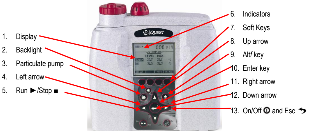
Figure 2-2: EVM keypad and display explained
