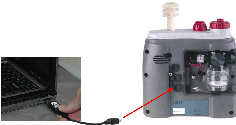
Figure 2-7: Communicating with DMS via USB cable
