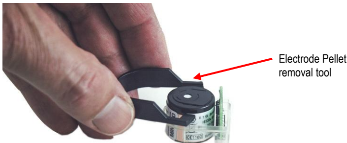
Figure 7-3: Removing the lamp with removal tool
