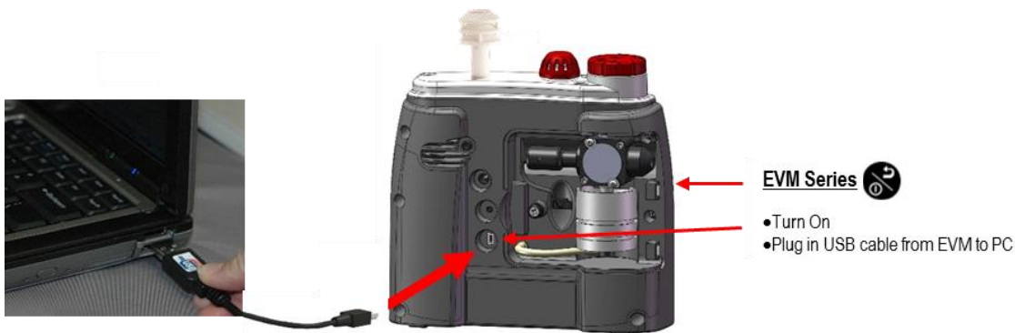
Figure 6: Communicating with the Environmental Monitor and Detection Management Software
