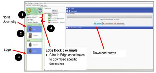
Figure 5-3: Downloading in DMS with the Edge
