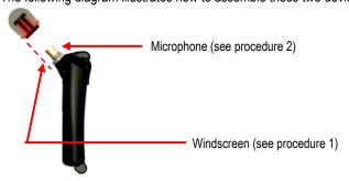
Figure 6-1: Microphone and windscreen assembly
