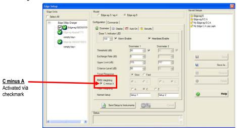
Figure 3-8: C-A measurement setup
