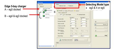
Figure 1-3: Parameter setup screen for Model eg5
