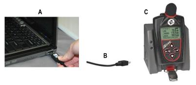
Figure 3-5: Communicating—connecting a docked Edge to a PC
