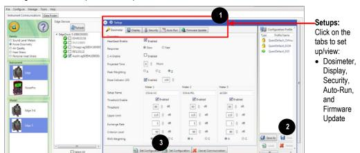
Figure 3-15: Saving and sending Edge setups
