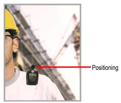
Figure 4-2: Attaching the Edge on your shoulder
