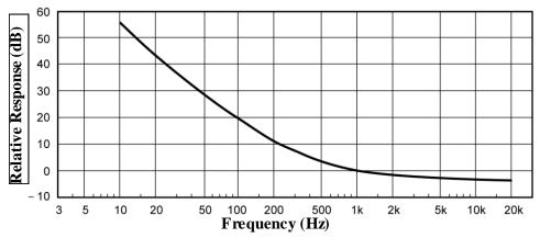
Figure B-1: C-A weighting response curve
