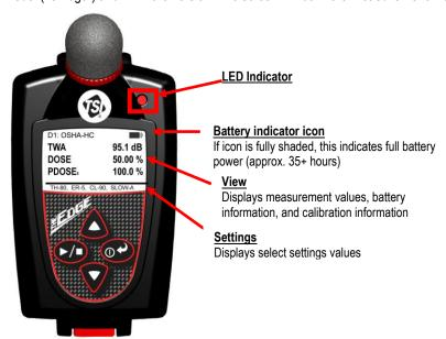
Figure 2-2: Powered on with measurement view displayed
