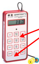
Figure 1-171: QUESTemp° II keypads
