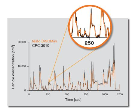
Compared to a CPC, testo DiSCmini is truly handheld, easier to use and it delivers not only the particle number concentration but also average particle diameter and lung-deposited surface area. testo DiSCmini measures size particles smaller than about half a micron in diameter.
