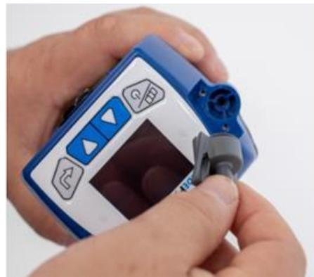
2. Flip the instrument upside down to remove the impactor disk.
