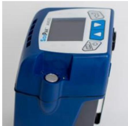
6. Place inlet gasket on the inlet so that the tabs on the gasket fit inside the inlet around inner tabs of the inlet as shown.
