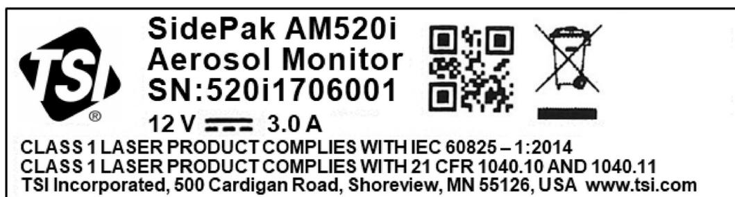
There are no user-serviceable parts inside this instrument. Performing services other than those described in this manual may result in exposure to harmful (visible) laser radiation. A warning label like the one shown below is affixed to the internal laser device.
