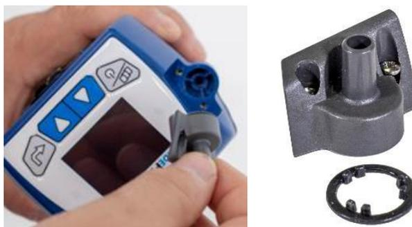
2. Attach the Dorr-Oliver cyclone to the DPM cyclone to create the DPM assembly.
