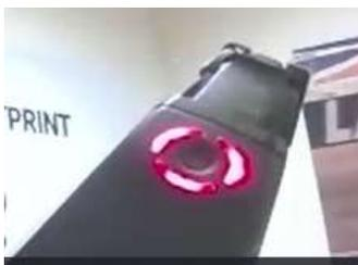
When the instrument is emitting X-rays, the light on top will be blinking red.
