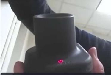
It comes with a wall charger. The charger light is red when it is plugged in and empty.
