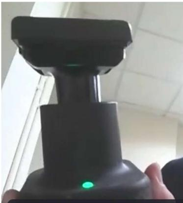
When the battery is plugged in, the light blinks green when it is charging, and it is solid green when it is done charging.
