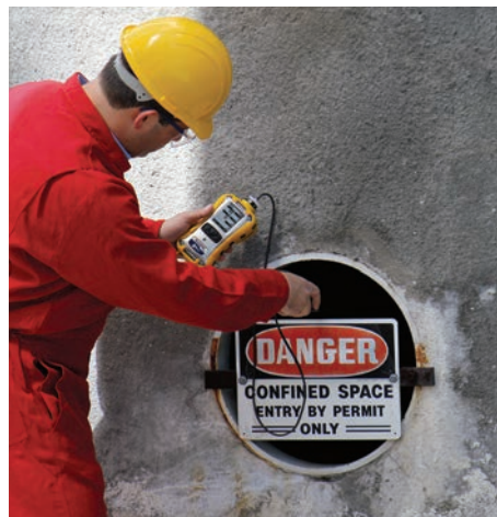
Confined space testing with the MultiRAE Lite
