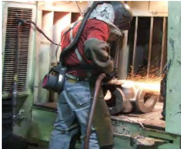
A worker grinding castings in a foundry. The work is performed in a ventilated booth to reduce the worker's exposure to silica.
